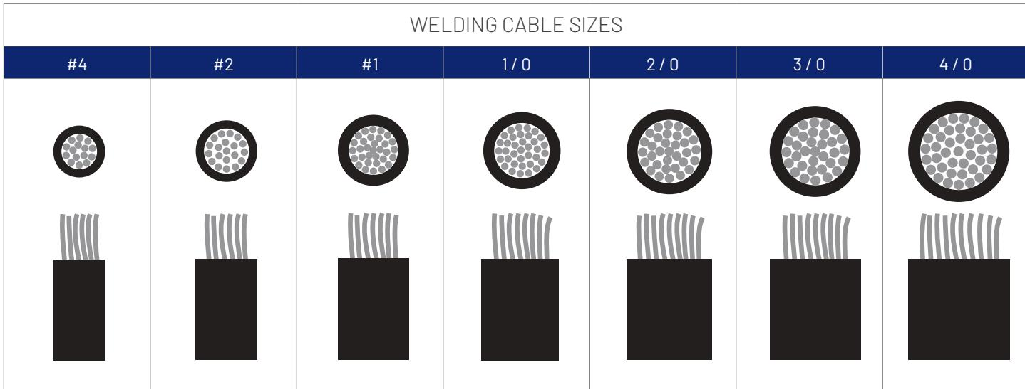
NOTE 1: Welding cable sizes are drawn to scale.
