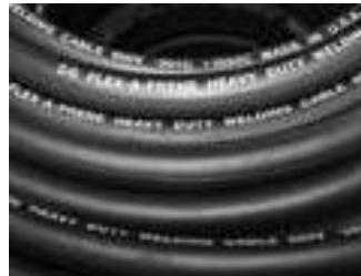
Direct integrates Quick Print® capabilities into its long- and short-run manufacturing processes allowing customizable ink printing along the outer cable jacketing to help company branding, identify cable types, and deter theft.
